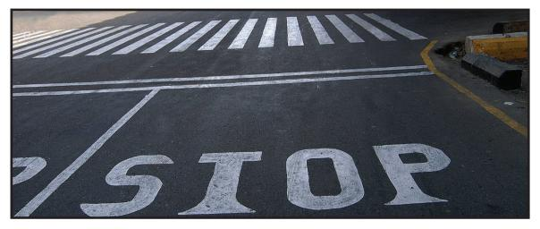
• A stop line is a single, solid, transverse line painted before the intersecting edge of the road junction/intersection.
