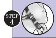
**Buckles -** Centre the left buckle under the chin. On most helmets, the straps can be pulled from the back of the helmet to lengthen or shorten the chin straps. This task is easier if you take the helmet off to make these adjustments.
